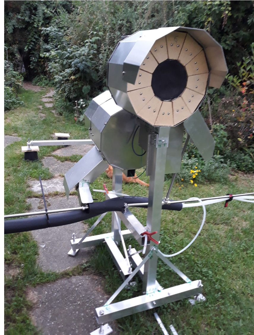
Receiver of Reflector – Solar Thermal
